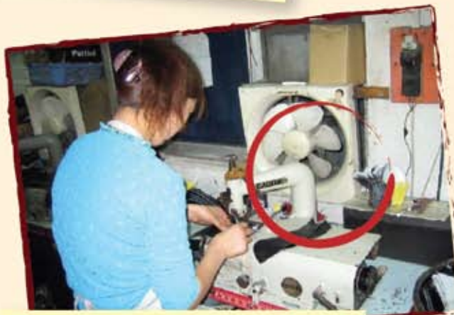
The factory set up individual 'ventilation systems' following suggestions made by workers, and regularly checked and cleaned the exhaust fans to ensure the effective removal of dust from the workplace.
